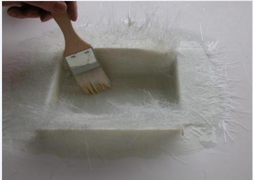
With the use of a brush, saturate fibreglass cloth with resin. Use a lamination roller to remove air bubbles and excess resin.
